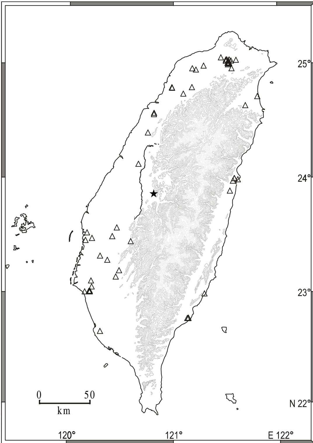
Figure 4. Locations of the CWB real-time strong-motion arrays in buildings and bridges. The "star" indicates the location of the main shock. Surface ruptures extending about 80 km north-south are shown to the left of the main shock.
