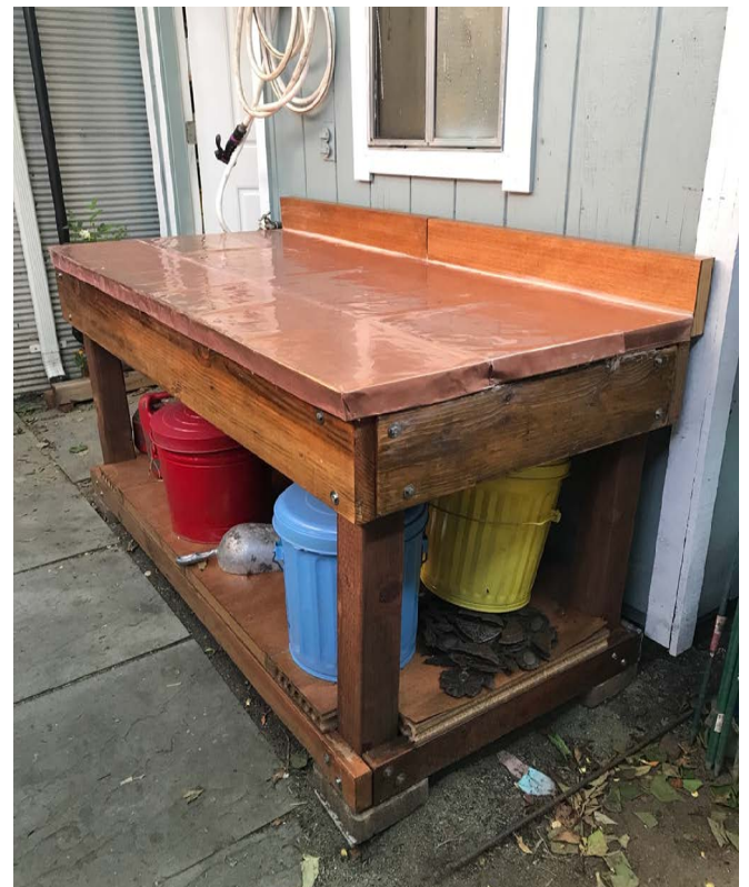
copper top. I later fastened it with bronze boat nails and calked it
